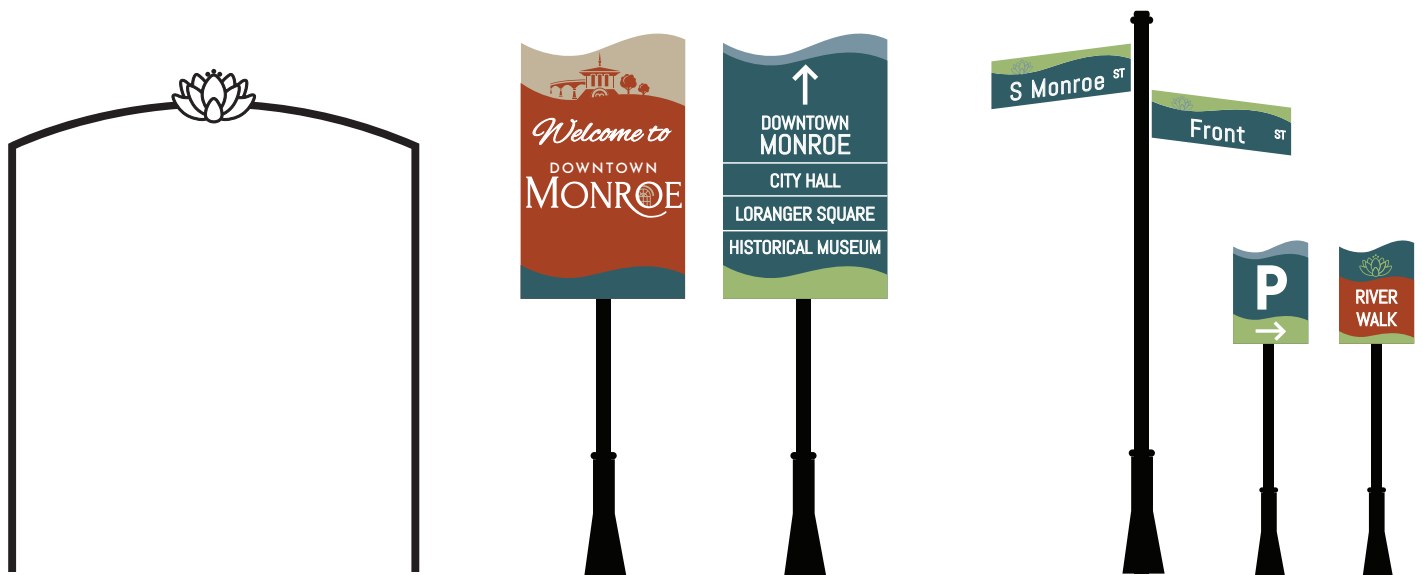
Figure 22: Alley archways with fabricated metal [left]. District and directional signs with painted metal and reflective vinyl (City of Monroe)
